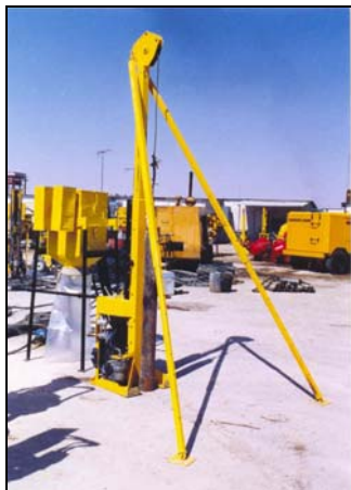
Fig-3: Drop Hammer Rig
