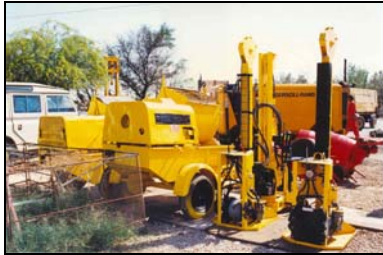
Fig-1: Minipiling Equipment
